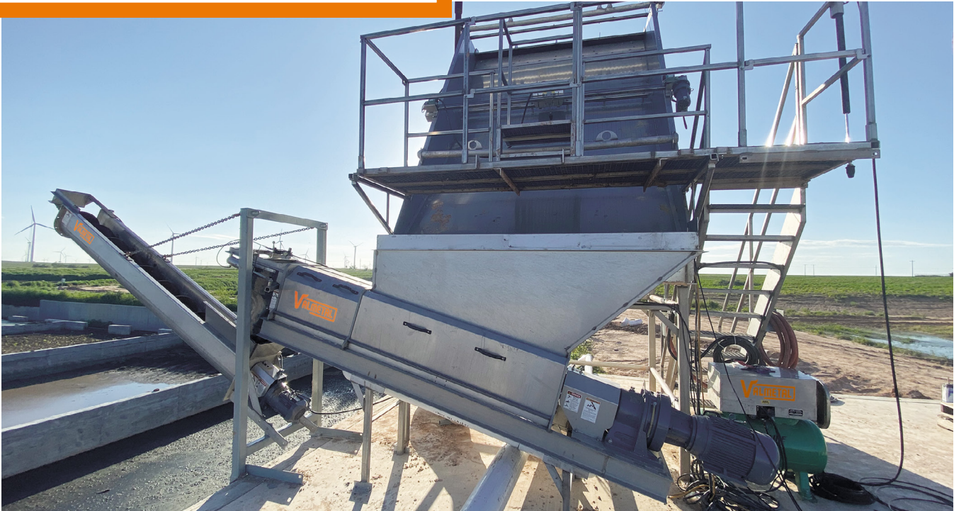
Our on-board vibrator increases capacity and helps keep screens clean.
